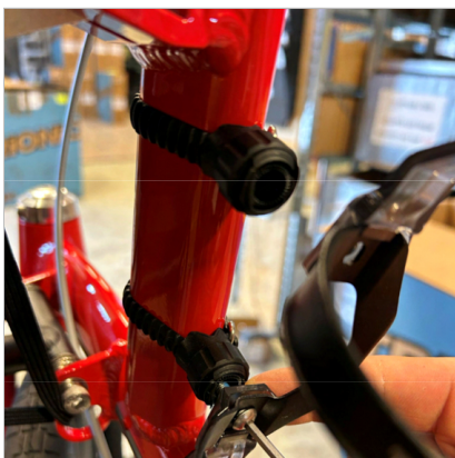
⑦ Attach the bottle holder with the two screws. The "opening" of the bottle holder should face outwards.
