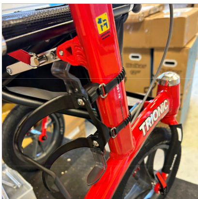
⑧ The bottle holder is now attached to the frame and you enter the bottle from the side and remove it outwards.
